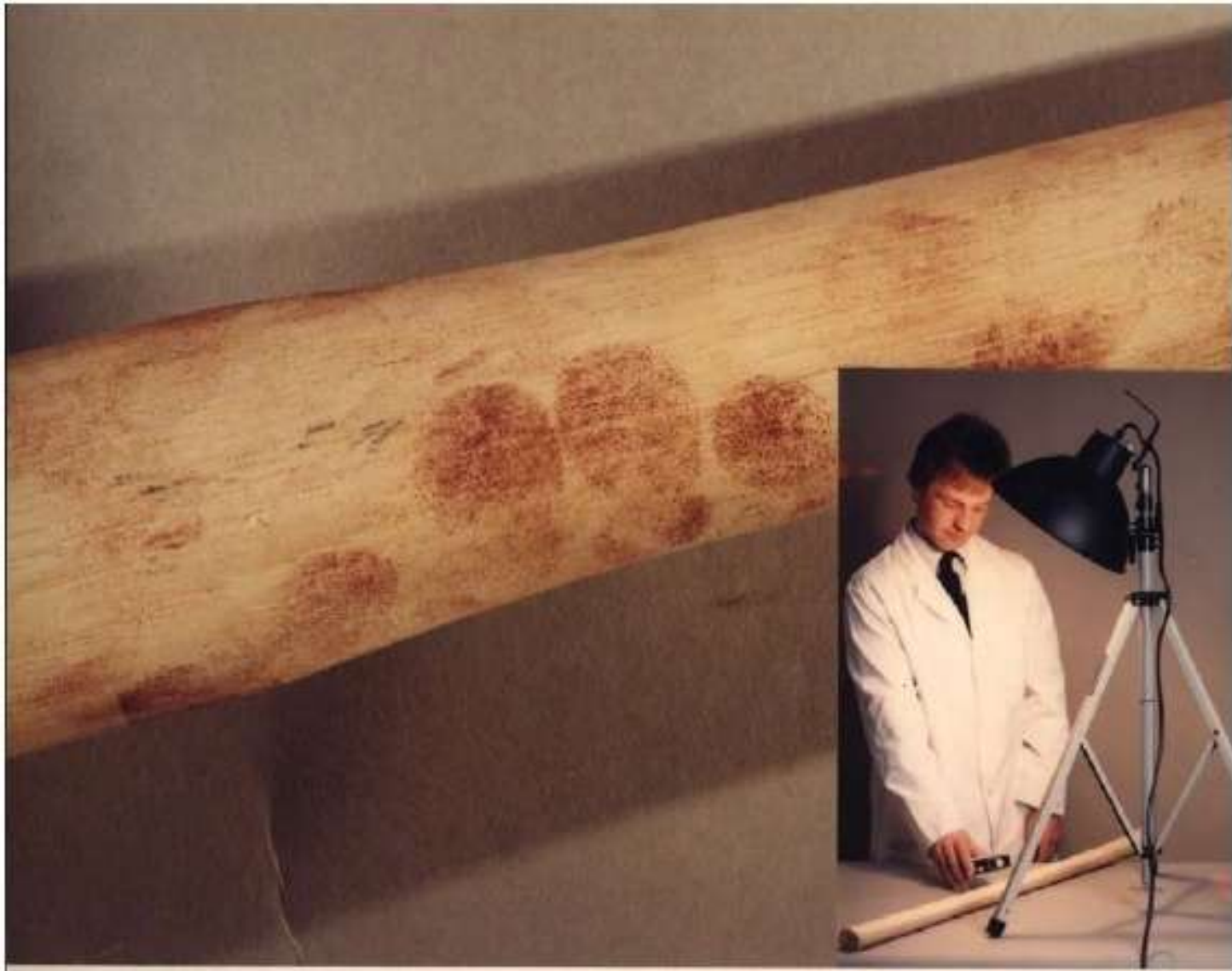
SILVER NITRATE developed fingerprint. Inset: illuminating to develop fingerprints
