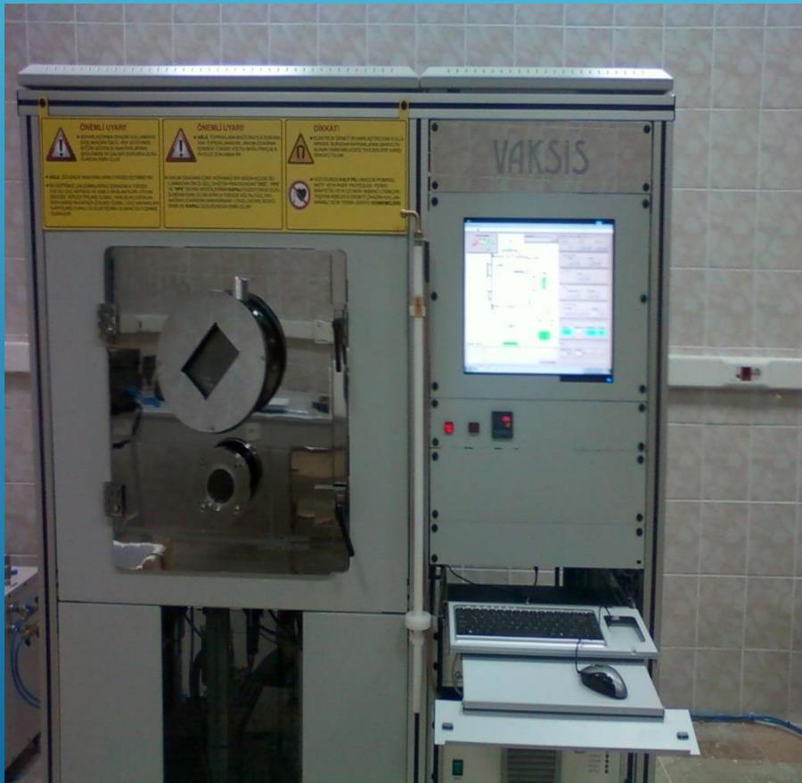
In our laboratory; binary, ternary and quaternary semiconductor thin films belonging to II-VI, I-III-VI, II-III-VI and I-II-IV-VI groups are produced by **E-beam** and **thermal evaporation techniques** and their electrical and optical characterizations are determined.
